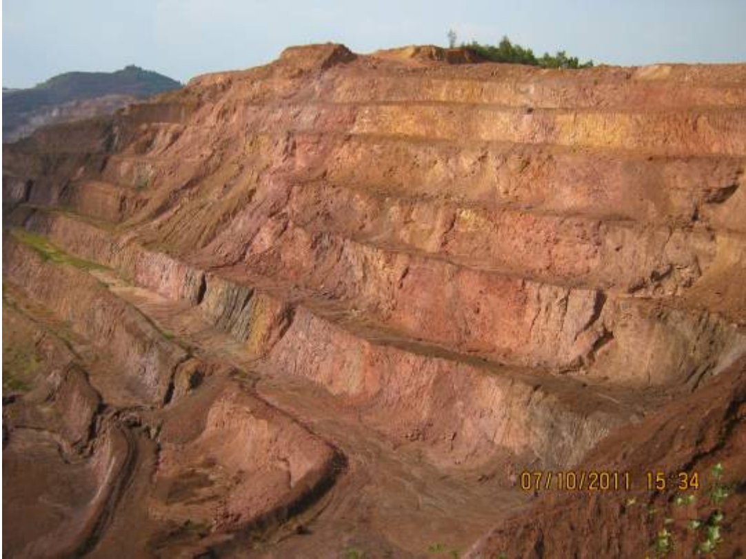
Sliding of mine benches due to unscientific mining of Sesa Goa mines of Chitradurga
