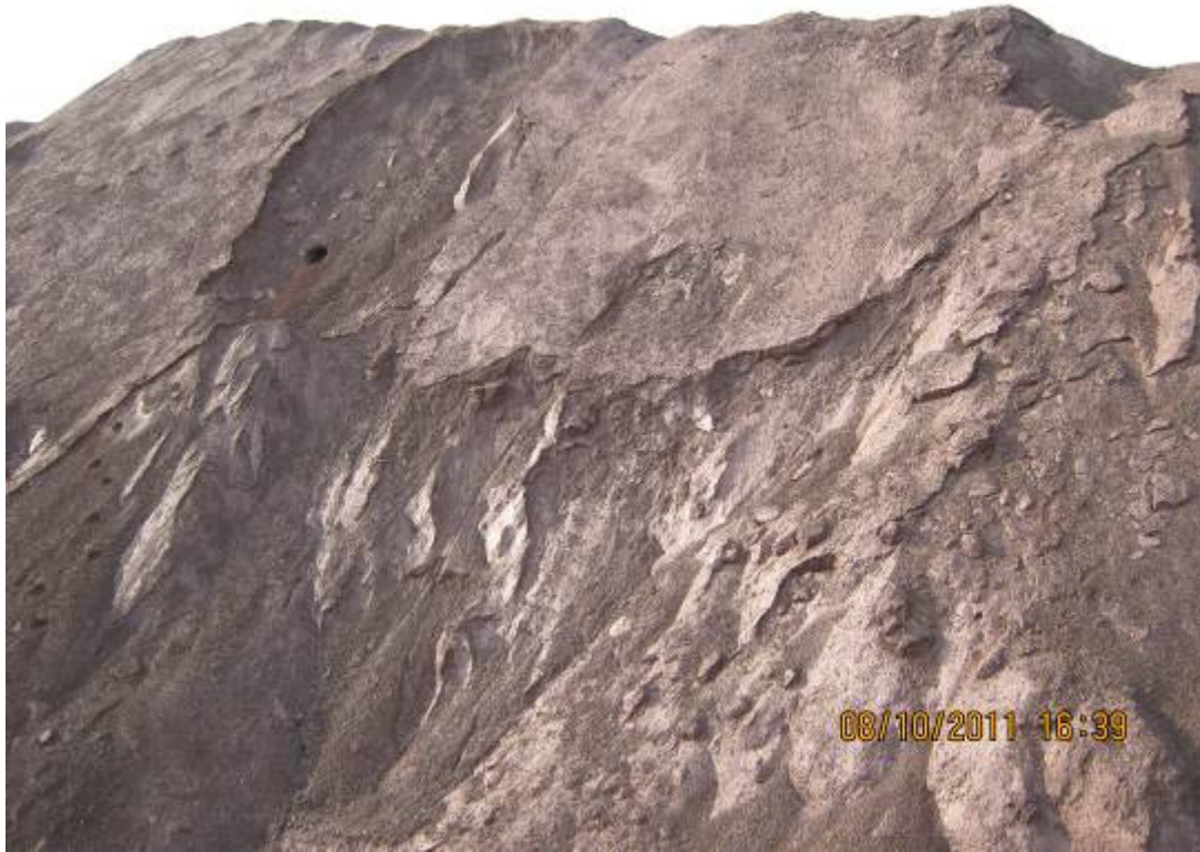
Erosion and improper stacking of fine ore material of Laxmi Narasima mines of Chitradurga
