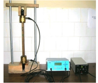
Ultrasonic Wood Tester to detect defects in wood
